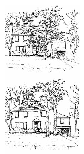
**Figure A.6**. Trees south of a home before and after pruning. Lower branches are pruned up to increase heat gain from winter sun (Sand 1993).
