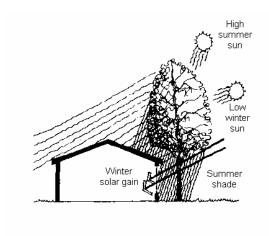
**Figure A.5**. Select solar-friendly trees for southern exposures and locate them close enough to provide winter solar access and summer shade (Sand 1991).
