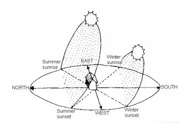
**Figure A.3.** Paths of the sun on winter and summer solstices (Sand 1991). Summer heat gain is primarily through east- and west-facing windows and walls. The roof receives most irradiance, but insulated attics reduce heat gain to living spaces. The winter sun, at a lower angle, strikes the south-facing surfaces.
